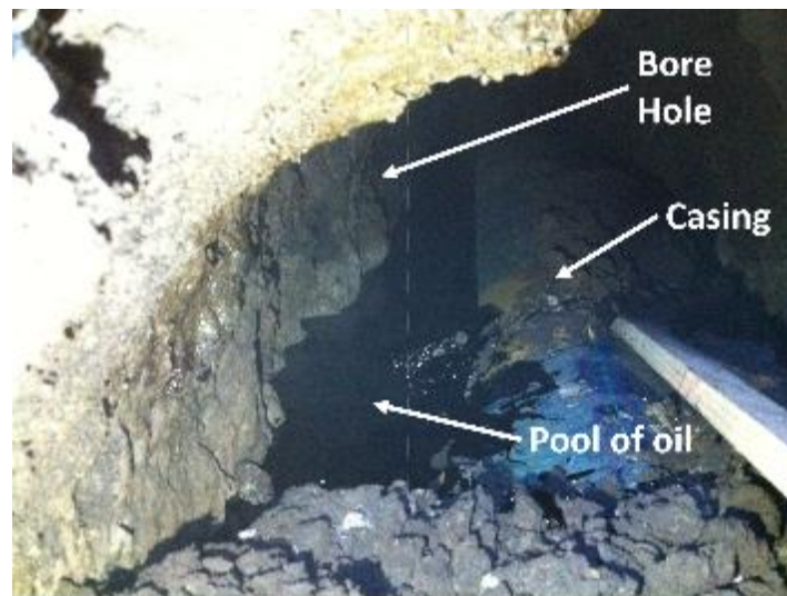
Figure 23: View at the borehole entrance accompanied by audible fluid sounds emanating from the opening
