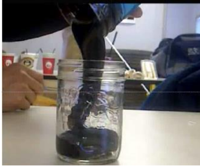
Figure 24: Sample from the borehole entrance transferred to another container. Sample temperature at the pour time was 4.5°C (40°F)
